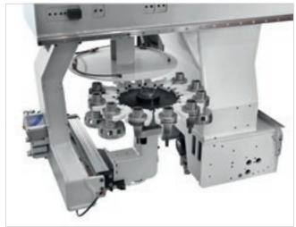
Revolver magazine with 12 overhead positions and 12 on the X carriage, reducing cycle times to the minimum.
